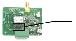
Relay mode can be changed by jumper N.O / N.C
