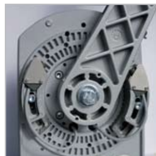
Adjustable mechanical and electronic limit switches in opening and closing
