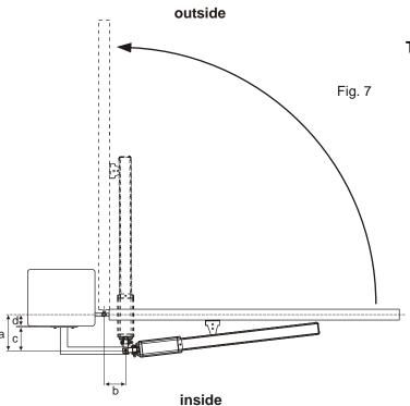
Total stroke 270 mm - max suggested stroke 250 mm
