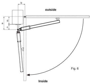
Total stroke 270 mm - max suggested stroke 250 mm
