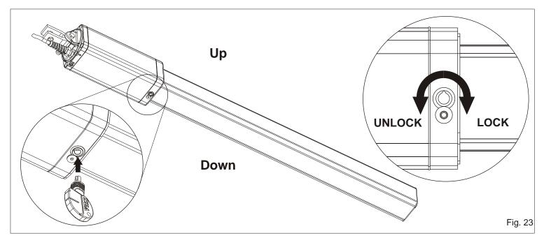
**WARNING:** SEA recommends to the end user to release the operator only after having switched off the electric power.
