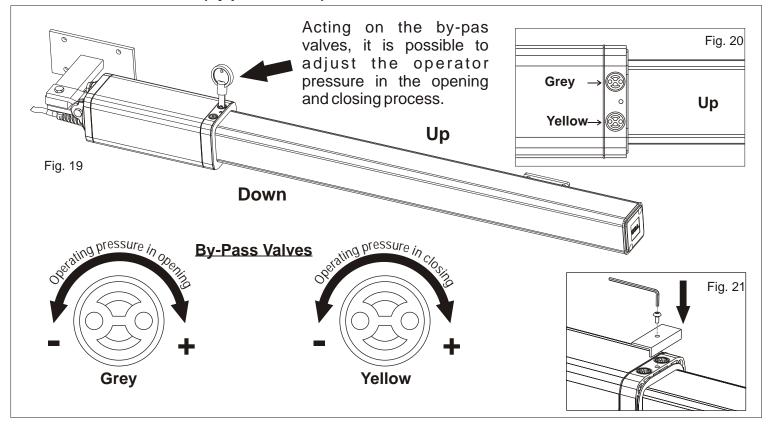
Adjust the opening and closing forces of the gate so that the diagram of the force is respected (present in the regulation EN 12453); Anyway the max. thrust force should never be superior of 15 KgF.
